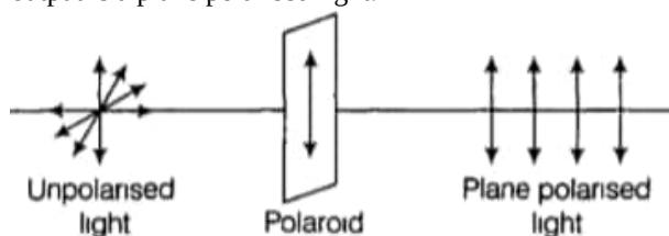
ii. Intensity coming out of a single polaroid is half of the incident intensity so, the intensity of transmitted light from polaroid  $P_1$ ,  $I = \frac{I_0}{2}$
