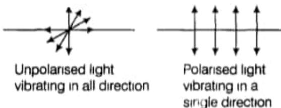
Polaroid is a special crystalline solid which contains a special axis called the optic axis. When we make an unpolarised light to fall on a polaroid. Only vibration parallel to optic axis is allowed to pass through and all other vibration are cut. Thus, the output is a plane polarised light.
