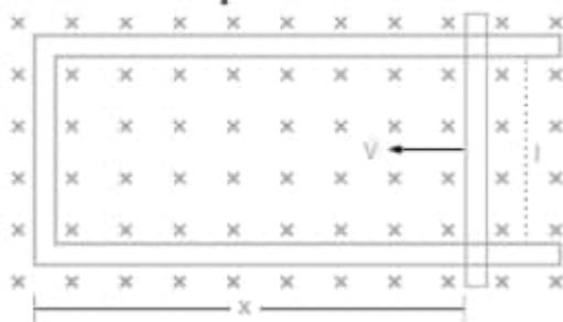
ii. How does one understand this motional emf by invoking the Lorentz force acting on the free charge carriers of the conductor? Explain.
