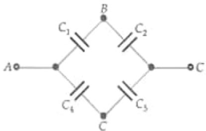
Capacitors  $C_1$  and  $C_2$  form a series combination of equivalent capacitance  $C_6$  given by
