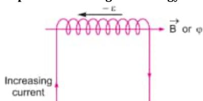
When a time varying current flows through the coil, back emf ( $-\varepsilon$ ) produces, which opposes the growth of the current flow. It means some work needs to be done against induced emf in establishing a current  $I$ . This work done will be stored as magnetic potential energy.
