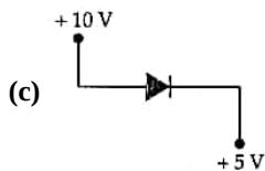
**Explanation:** The p-side is at higher potential (+10V) and n-side is at lower potential (+5V).
