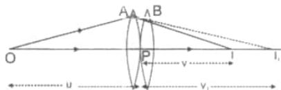
Two thin lenses, of focal length  $f_1$  and  $f_2$  are kept in contact. Let  $O$  be the position of the object and let  $u$  be the object distance. The distance of the image (which is at  $I_1$ ), for the first lens is  $v_1$
