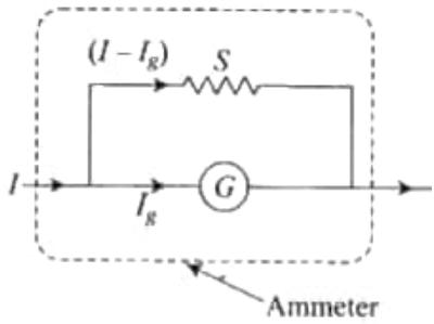
For measuring  $I_1 = 10 \text{ mA}$  :  $I_g \cdot G = (I_1 - I_G)(S_1 + S_2 + S_3)$
