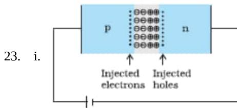
During the formation of p - n junction diode; due to the concentration gradient across p and n sides of a diode, holes diffuse from p side to n side and electrons diffuse from n side to p side giving rise to development of immobile positive charges on the n side and the negative charges on the p side across the junction. Thus a potential barrier is formed at the junction.
