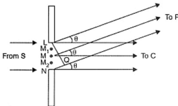
We, therefore, get maxima and minima, i.e., a diffraction pattern, on the screen. **Maxima and minima** are produced when the path difference between waves is a whole number of wavelengths or an odd number of half wavelengths respectively.
