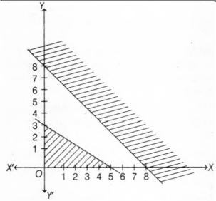
It can be concluded from the graph, that there is no point, which can satisfy all the constraints simultaneously. Therefore, the problem has no feasible solution.
