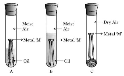
List your observations in each of the three cases A, B and C with reason, if the metal 'M' is generally protected against corrosion by the method of galvanisation.
