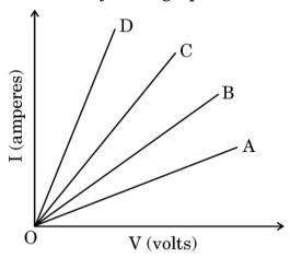
(a) Which one of the graphs represents the series combination of  $R_1$  and  $R_2$ ?
